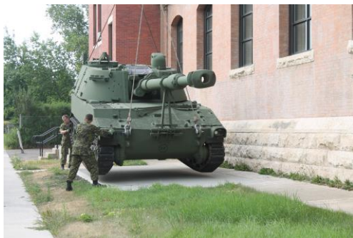
The Rigging Team lines up the M-109 on the landing marks; Photo SDI
